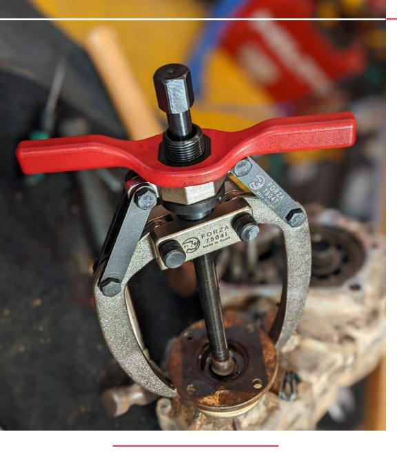
Wide range of pullers for external applications. Specially designed to remove bearings, pulleys, gears, axes and many other mechanical parts.
